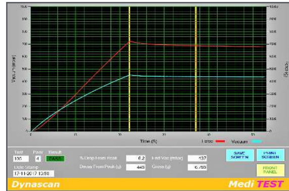
Display of the test results for a selected sensor position, showing good seal integrity for the test strip packs in question.
