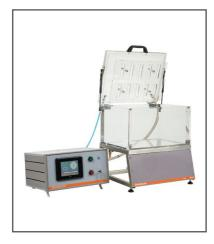
The system is programmed from a colour touchscreen display for method development and can then be locked to prevent unauthorised changes. Automatic test cycles are initiated by a simple press of the start button. The display will indicate the end of the test cycle. In the case of altitude simulation, ascent and descent profiles can be displayed graphically.
